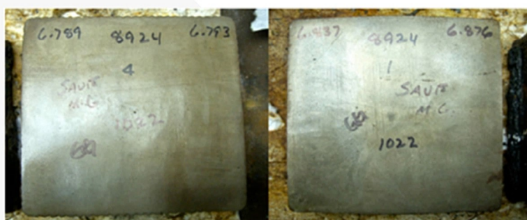
Fig. 3 First WAVE billet samples. #4 is WAVE (left) and #1 is Control (right)
